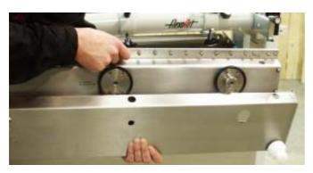
**Truly ink tight** - a "dual chamber" configuration in stainless steel ensures dripless ink metering.
