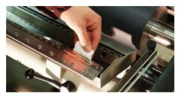
**Quick and easy change of blades**- due to unique GripTite® doctor blade system.
