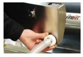
**Quick connector** - for easy tube connection and fast release of ink.
