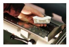
**Long life end-seals** - cost efficient and easy to exchange.
